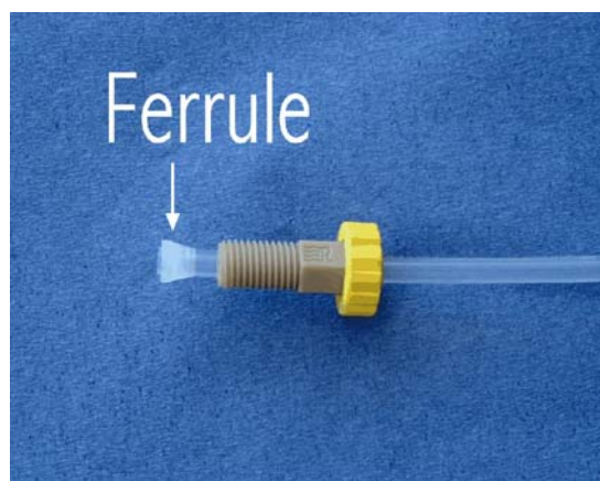
Fitting with correct position of the ferrule
